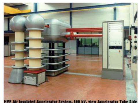
HVE Air Insulated Accelerator System, 500 kV, view Accelerator Tube Side
