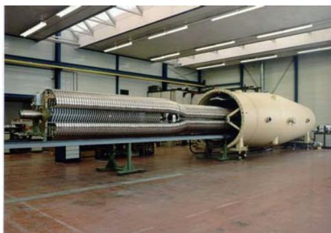
HVE 5.0 MV Tandatron Accelerator System, detail interior rolled out
